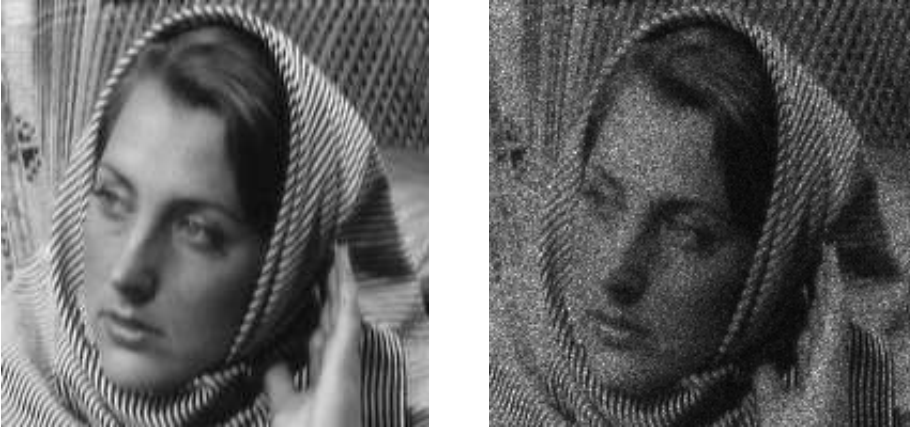
Figure 3: Left : Original image. Right : Noisy image corrupted with Gamma noise of standard deviation 0.2.
