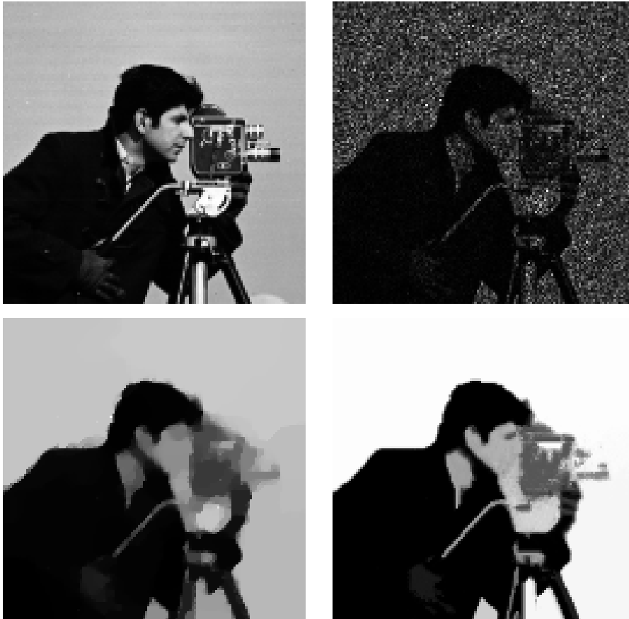
Figure 6: Top: Original 'cameraman image' (left) and corrupted image by multiplicative Gamma noise of standard deviation 0.5 (right). Bottom: Restored image by the I-divergence - TV model with \lambda = 0.9 (left) and the result by one iteration of the I-divergence - NL-means model with \lambda = 0.6 , a = 1.5 , p = 5 , \omega = 21 and \tilde{m} = 5 (right).
